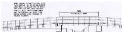
Fig. 2: Proposed elevations - 'Glentrool' type footbridge
